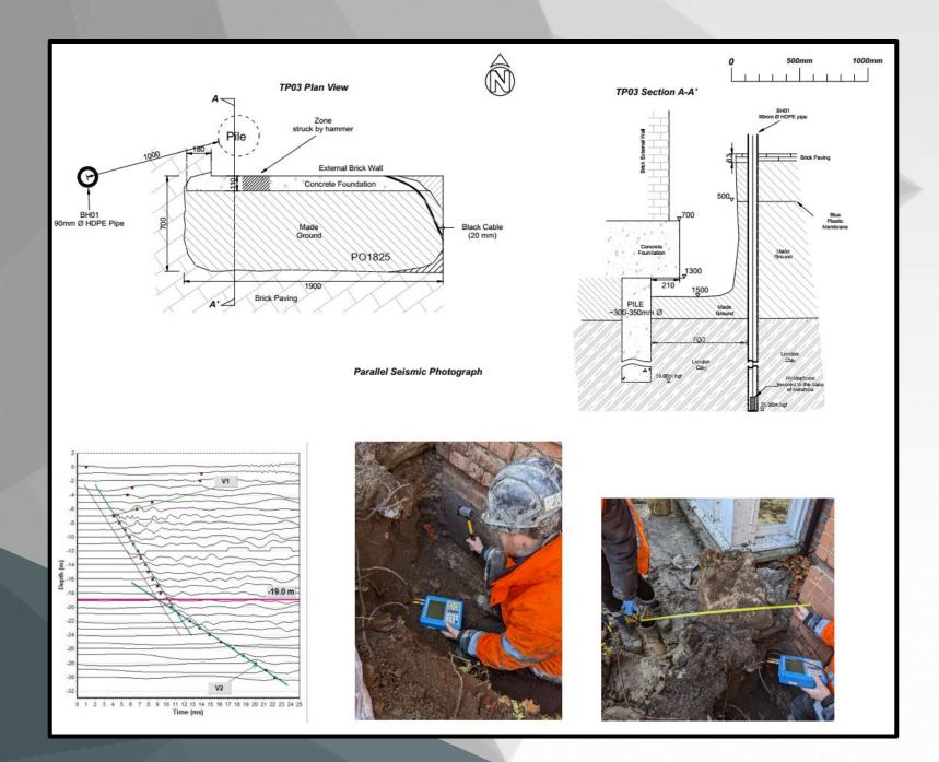
Where pile length data is required, our engineers use parallel seismic analysis to record the speed of P Wave arrival through the pile element. The seismic waves are generated by striking the foundation with an instrumented hammer and captured by an hydrophone receiver positioned in an adjacent test borehole.
