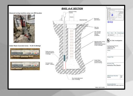
Where required, intrusive techniques can be used such as pile probing and coring, to confirm pile lengths and recover samples for detailed inspection and laboratory analysis.
